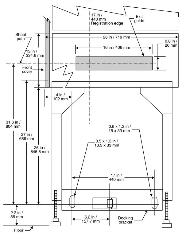
Figure 6-7. Bypass transport dimensions
